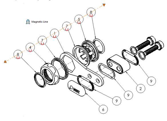
AutoBalloon - Automatically assigns balloons to all components (but does not assign balloons to the parts that are the same).
